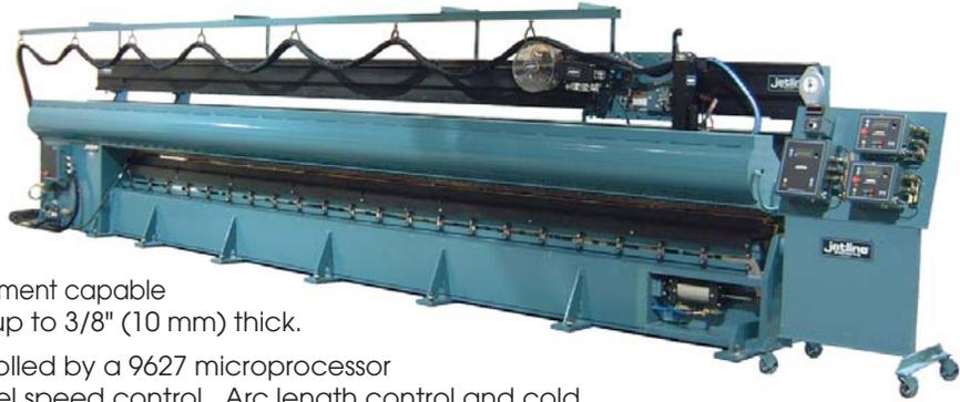
The welding procedure is controlled by a 9627 microprocessor control providing precision travel speed control. Arc length control and cold wire feed are included. The complete welding process is monitored and controlled at the operator control station. Video monitoring can be included to provide the operator with a clear view of the welding area throughout the complete weld process.
