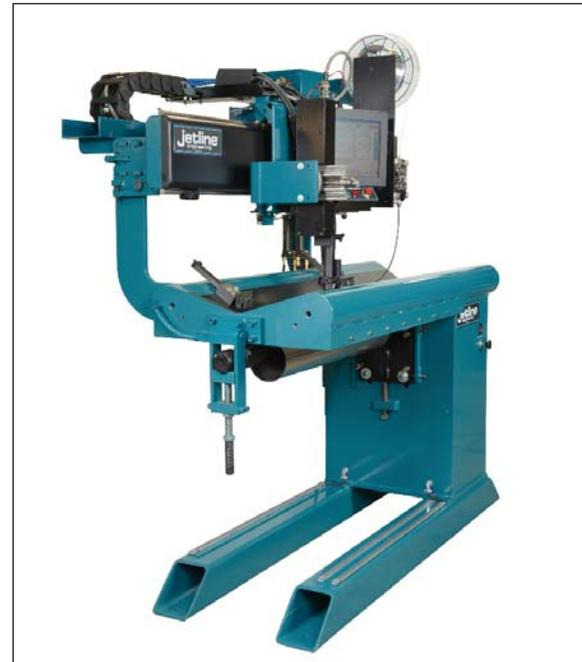
All Jetline seam welders use "chill-shunt" tooling which absorbs and dissipates heat through the use of additional mass operating under pressure against the work piece in the weld zone.
