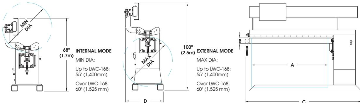
Combination seam welders are supplied with a removable riser which increases the diameter of parts that can be accommodated underneath the tabletop. Removal of the riser reduces the overall height of the machine. The tabletop is designed to allow internal welding as well.
