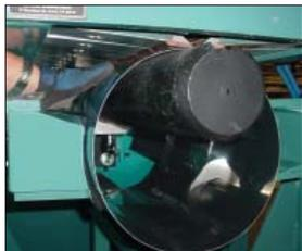
5. The pneumatic push-in cylinder moves in to close the gap between the edges of the part and to provide a gap free condition for welding. The hold down blade prevents one edge of the part riding up and over the other.
