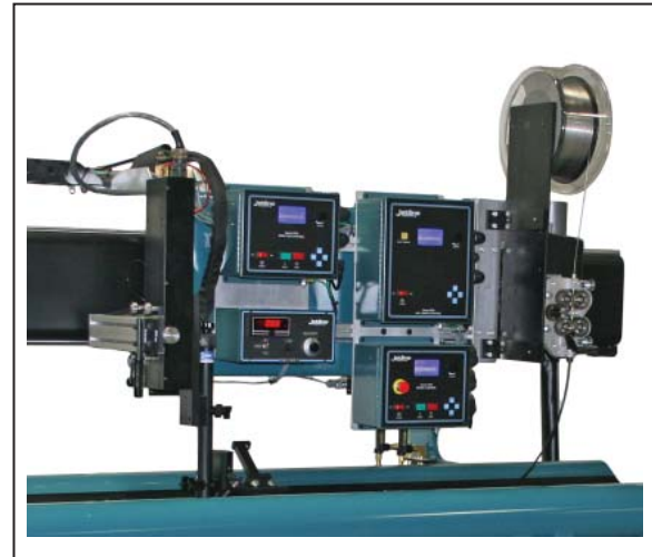
The 9700T travel control, 9700W wire feed control, and 9790 arc length control are shown mounted on a longitudinal seam welder carriage.
